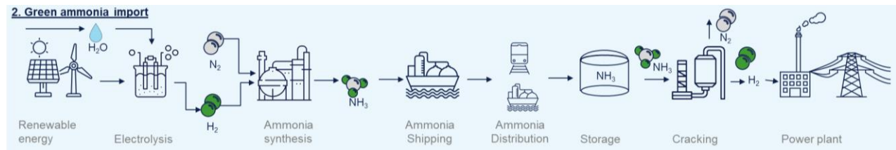
Figure 4: Process flow diagram of the green ammonia value chain.
